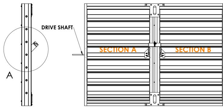
STEP 1: REMOVE EXISTING HEX NUTS AND WASHERS FROM U-BOLTS ON DRIVE BLADES. DO NOT REMOVE U-BOLT.
